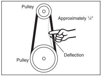
Figure 64. Checking the V-belt tension.
